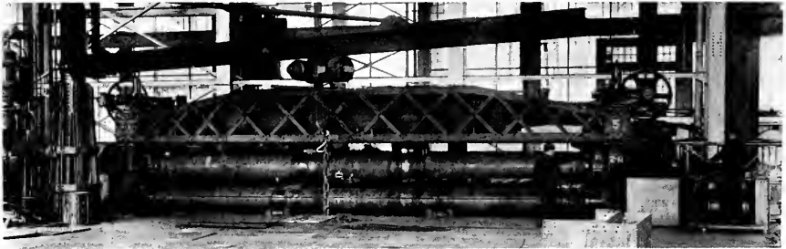
Fig. 1. A special self-supporting bracket crane, 3 tons capacity, 30-foot reach, used for serving what is said to be the largest bending rolls in the country. These rolls can cold bend plate 2 inches thick.
